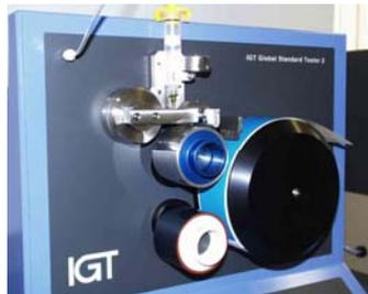
Fig.2: Damping unit GST2
