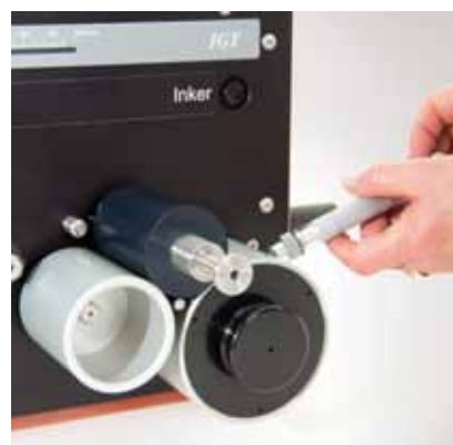
Applying ink with the IGT ink pipette
