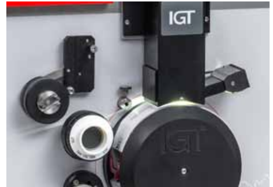
IGT Pick ISO 3783: the camera is scanning
