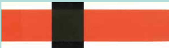
Flexo print on reference paper with black band for coverage, transparency, colour, density, etc.
