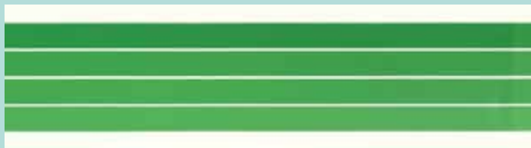
Flexo print of four bands to check the colour in four ink layers
