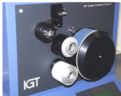
Fig. 1: Absorption of rubber blanket with Global Standard Tester 2
