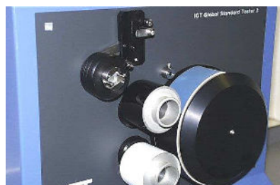
Fig. 1: Absorption of rubber blanket with Global Standard Tester 2
